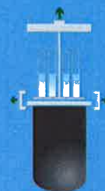
6 Clamp is released and sample rack automatically rises from chamber
